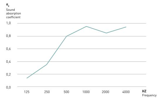
Weighted sound absorption coefficient:  $a_w = 0.65$  (MH)
